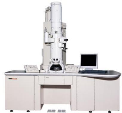
Electron beams are flows of electrons generated in the vacuum by heating or by applying a strong electric field to a fine filament, and have the nature of a "wave", with a wavelength shorter than that of visible light. Instead of glass, the lenses of an electron microscope are a combination of electromagnets constructed to form magnetic field lenses.
